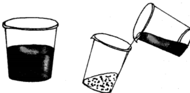
Fig. 5.11 Separating two components of a mixture by sedimentation and decantation.
